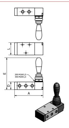
$\begin{array}{lll} A & = 100.5 \\ D & = 22 \\ E & = 90.5 \\ L & = 35 \\ Port & = G1/8" \\ Port \ exit & = G1/8" \\ Port \ supply \ and \ blowdown = G1/8" \end{array}$
